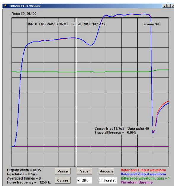
Figure 2.6.1 Input end waveforms with R1 = 100 Ohms and R2 = 200 Ohms
