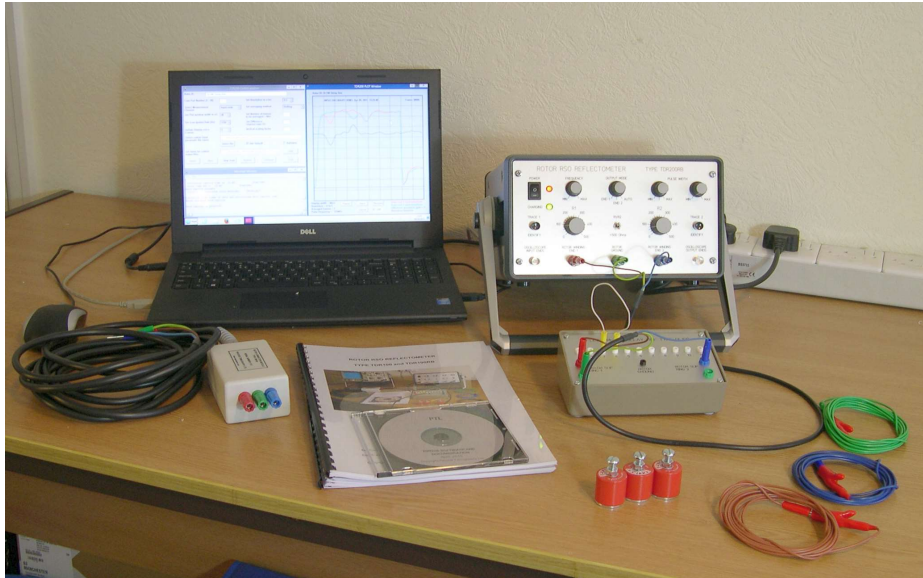
Figure 4.1(a) The TDR200 RSO Rotor Reflectometer measurement system in digital mode
